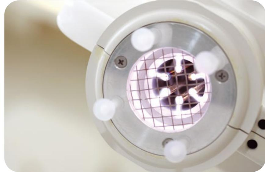
MicroPlaSter<sup>®</sup>; 2.45 GHz, 86 W, Ar 2.2 slm
